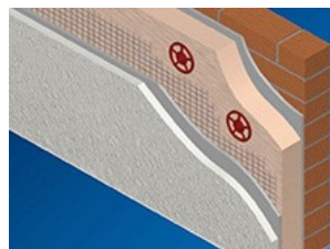
Layers of external wall insulation
